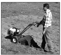
Figure 4-2: Guiding the tiller with one hand.
